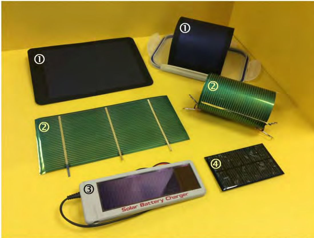
Fig 1. [LEFT] Commercial available solar cells. ① Amorphous silicon thin film, flexible; ② CIGS (Copper Indium Gallium Selenide), flexible; ③ amorphous silicon; and ④ polycrystalline silicon solar cells. [RIGHT] Rollable solar cell
