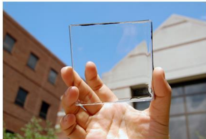
See-through solar-harvesting applications, such as this module pioneered at Michigan State University, have the potential of supplying 40 percent of U.S. electricity demand. Photo courtesy of Richard Lunt/Michigan State University
